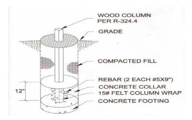
Post frame foundations shall be sized in accordance with RCO Table 324.3
