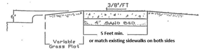
Concrete sidwalks to be four inches thick and saw cut every four (4) feet minimum.
