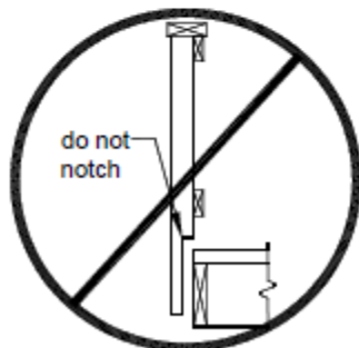
FIGURE 34: POST NOTCHES PROHIBITED
